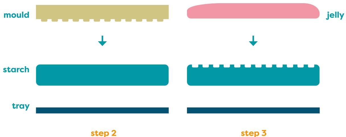
Figuur 1: Schematic representation of starch mould production
